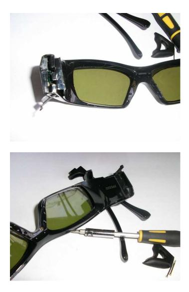
Once inside, the lenses on modern glasses seem often to be connected using a flexible PCB. On the SamSung glasses it was easy to solder the wires onto the solder pads connecting the lenses to the flex, then the control board was cut off to prevent it interfering. On the HiSense glasses, the wires had to be carefully soldered to the contacts at the end of the flex where it was meant to fit into a connector on the control board.
