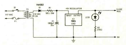
FIG. 3-REGULATED POWER SUPPLY is suitable for TTL and CMOS IC's.
