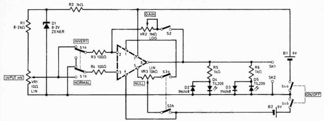
RECENTLY acquired a bulk purchase of i.c.s which contained many 741 series op-amps said to be untested. Looking through articles for the past couple of years failed to give any circuits for this purpose (although digital i.c. testers and transistor testers were fairly numerous). I therefore built the tester illustrated in Fig. 1, a simple circuit which has proved quick and easy to use as well as being relatively cheap.
