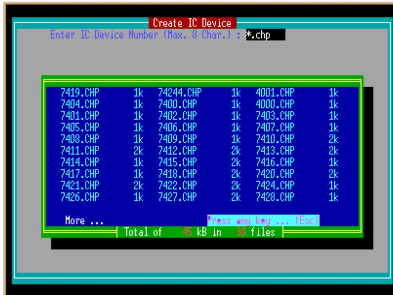
Then you will be asked for the pin quantity. IC that could be checked only which has pin quantity of 14-pins, 16-pins, 18-pins (seldom), 20-pins, 22-pins (seldom) and 24-pins. After that you will be asked for each of this pin whether it is an Input, Output, Clock, Vcc, Ground or Unused (not connected) pin. Select by inputting the number consecutively.
